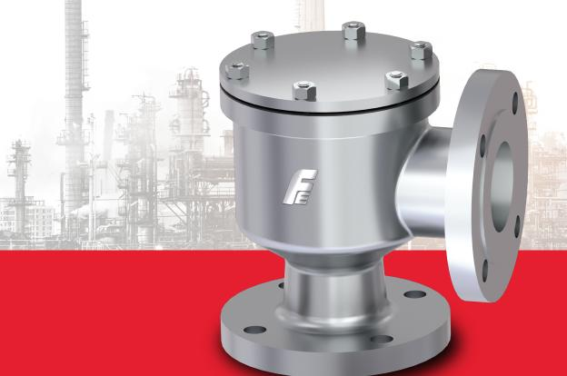
Pipe-Away Pressure Relief Vent is intended for use where pressure relief is required and the relieving vapors must be piped away and not vented to the atmosphere. A pallet in the vent housing opens and closes permitting relief necessary to avoid tank damage. A flanged side connection is provided for easy pipe-away of vapors eliminating the emission of vapors to the atmosphere.
